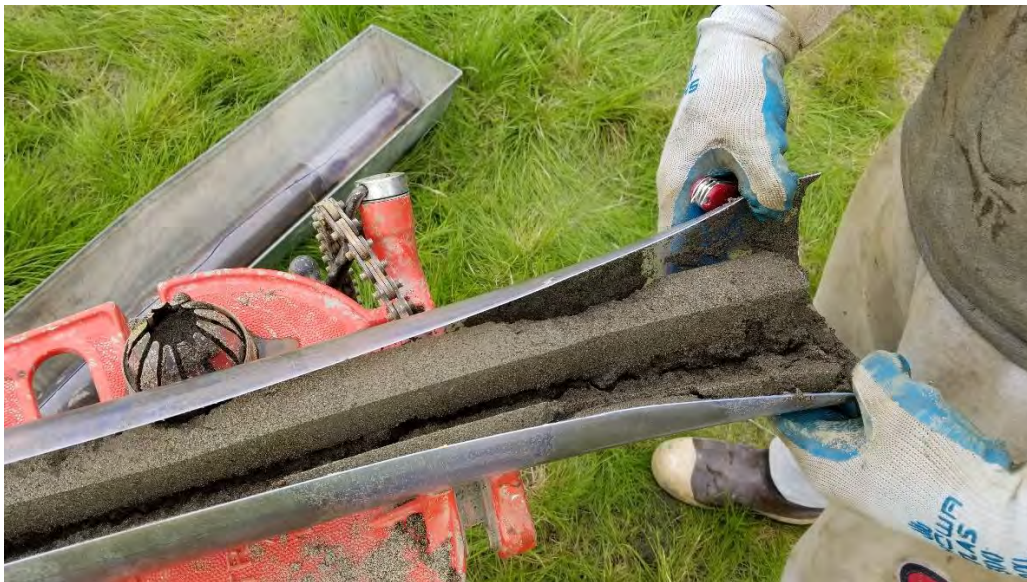
Photo No. 2 – 26 August 2019 The predominant soil type at the site was brown sand, such as this core from the 15-20 feet below ground surface interval from MW2A. View facing down.
