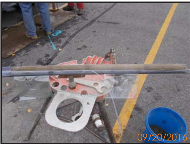
Photograph 3: Viewed Northeast- MW-3 and 4-8' soil profile.
