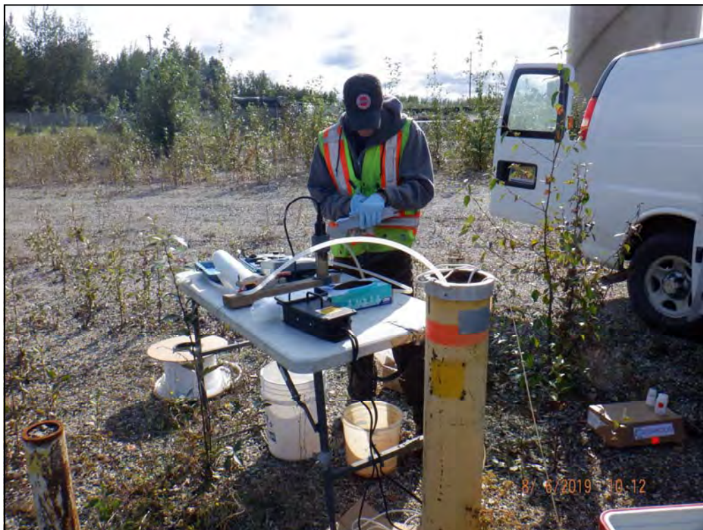
OU2 DRMO1 — Groundwater sampling at AP-10017R (view W)
