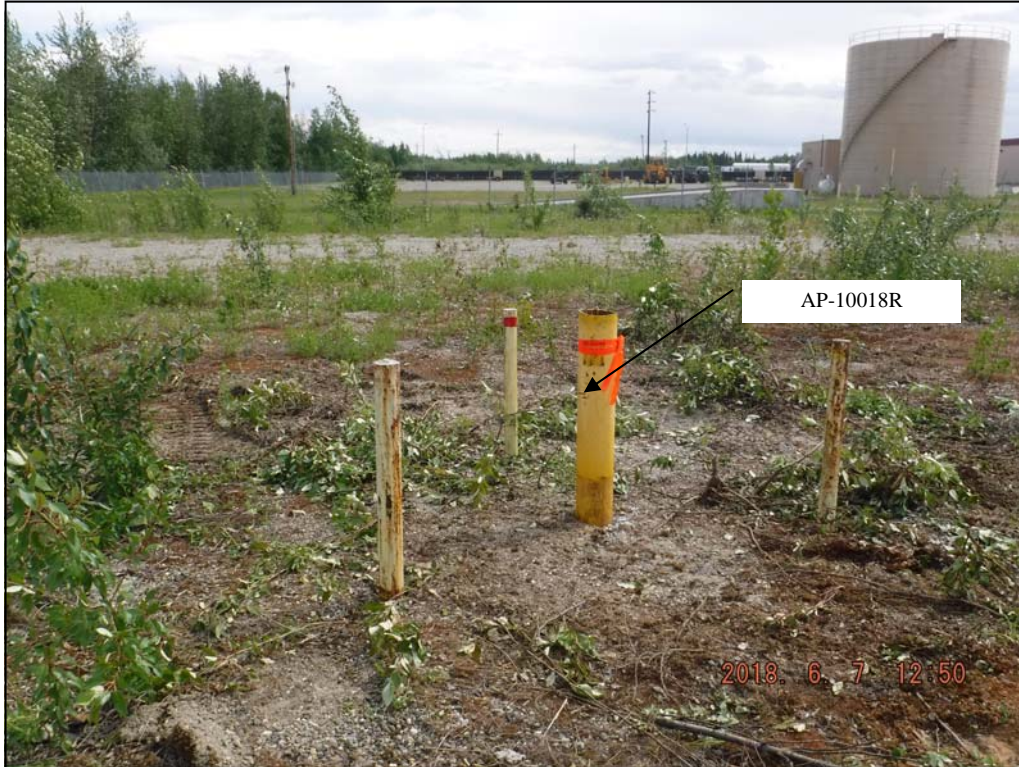
OU2 DRMO1 (3-Party) — Replacement Monitoring Well AP-10018R (view E)
