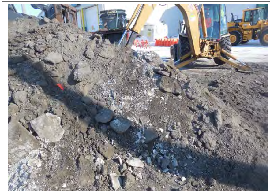
Photo 13: Field-screening samples were collected at 6-inches below ground surface at five locations in the soil stockpile, flagged by whiskers; looking north. (April 17, 2015)
