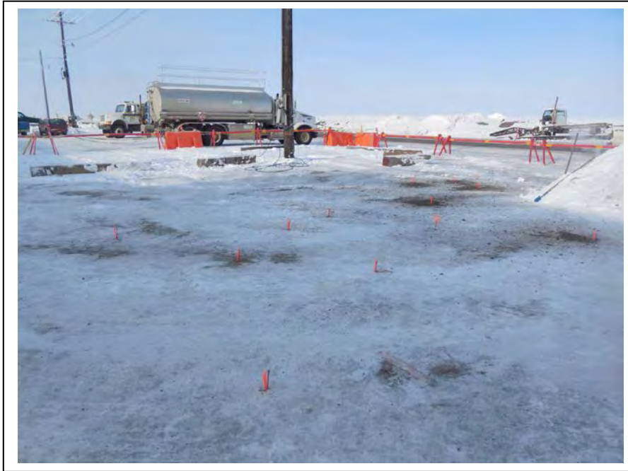
Photo 5: We field-screened surface soils at 14 locations in the fuel release (E1) area and six locations in the snow stockpile area (E2); locations marked with orange whiskers. (April 15, 2015)
