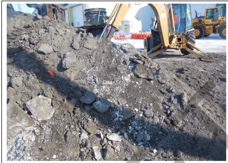
Photo 13: Field-screening samples were collected at 6-inches bgs at five locations within the soil stockpile. Locations were flagged with survey markers; looking north (April 17, 2015).
