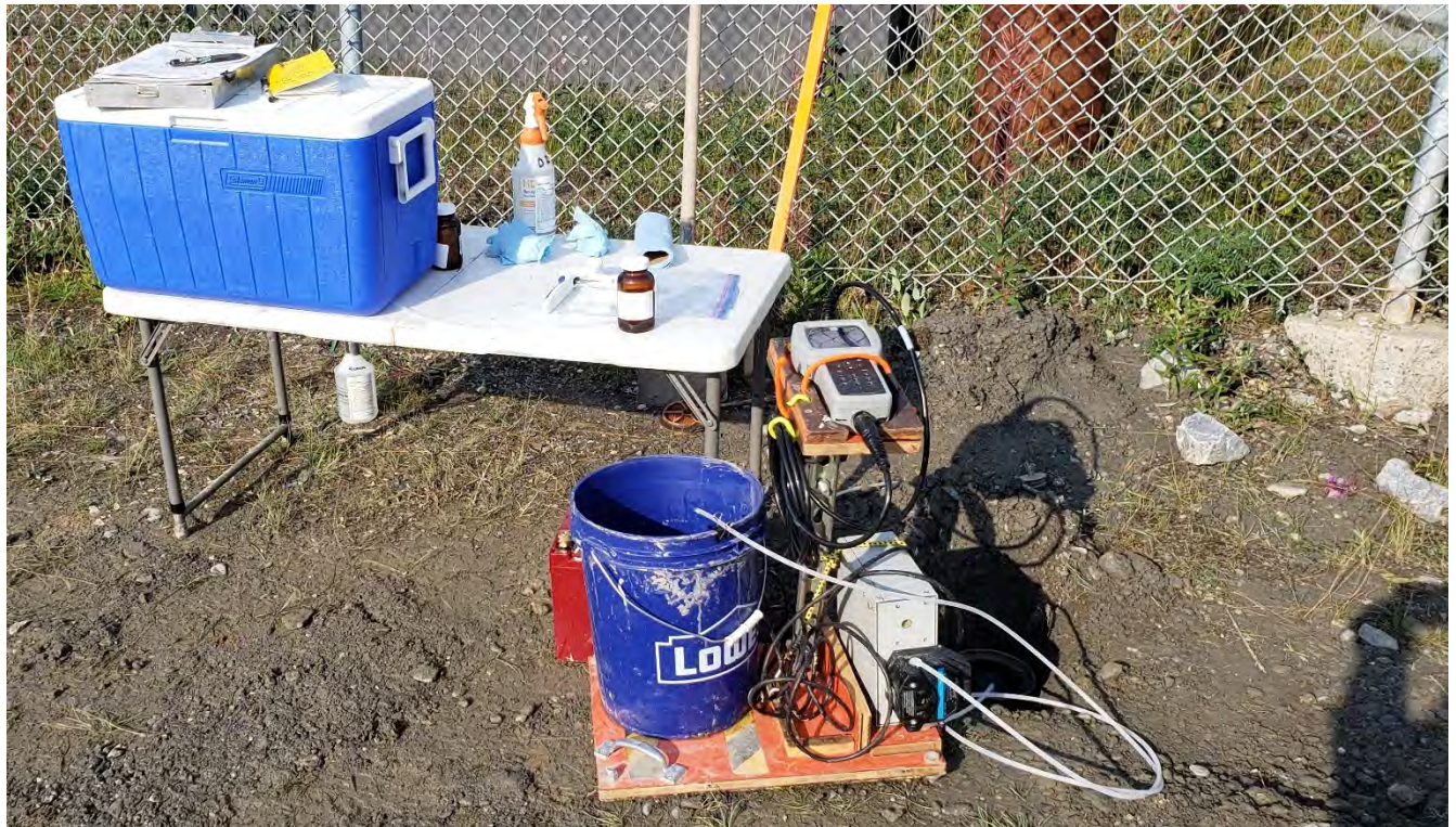
Photograph 6: Groundwater sampling at MW-193.
