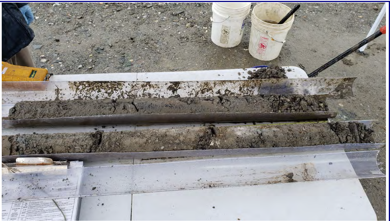
Photograph 3: MW-192 soil cores retrieved for soil logging and classification.
