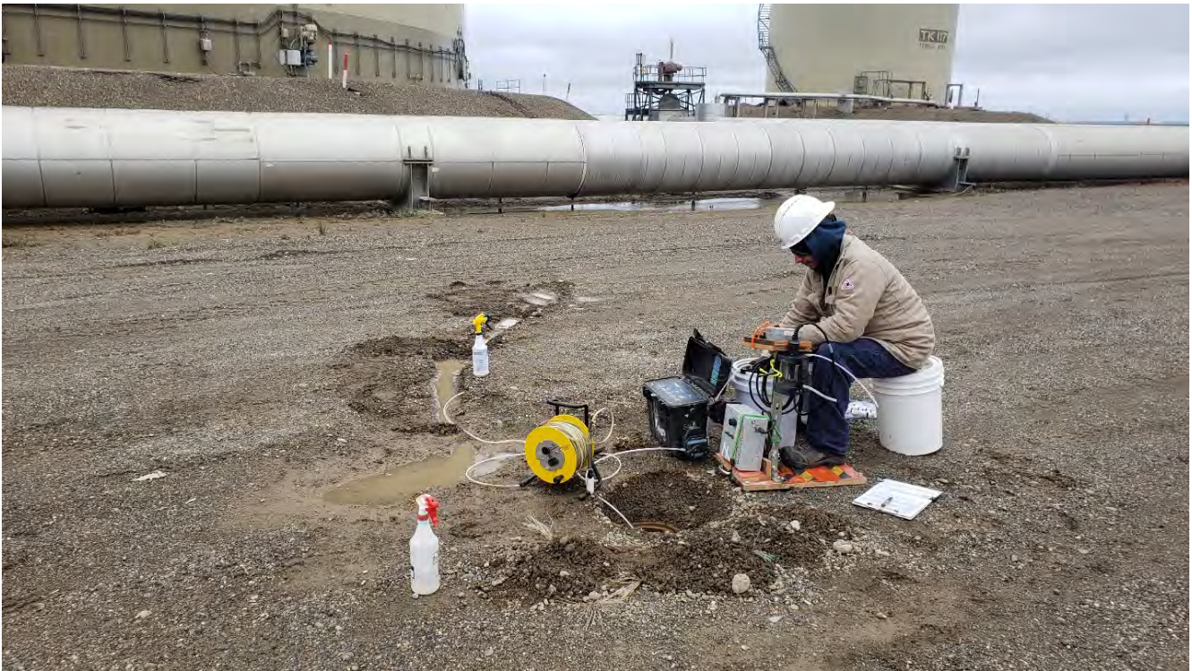
Photo 6: Monitoring Well MW-7R: A trench was created to direct ponded surface water away from the monitoring well during sampling, photograph facing north.
