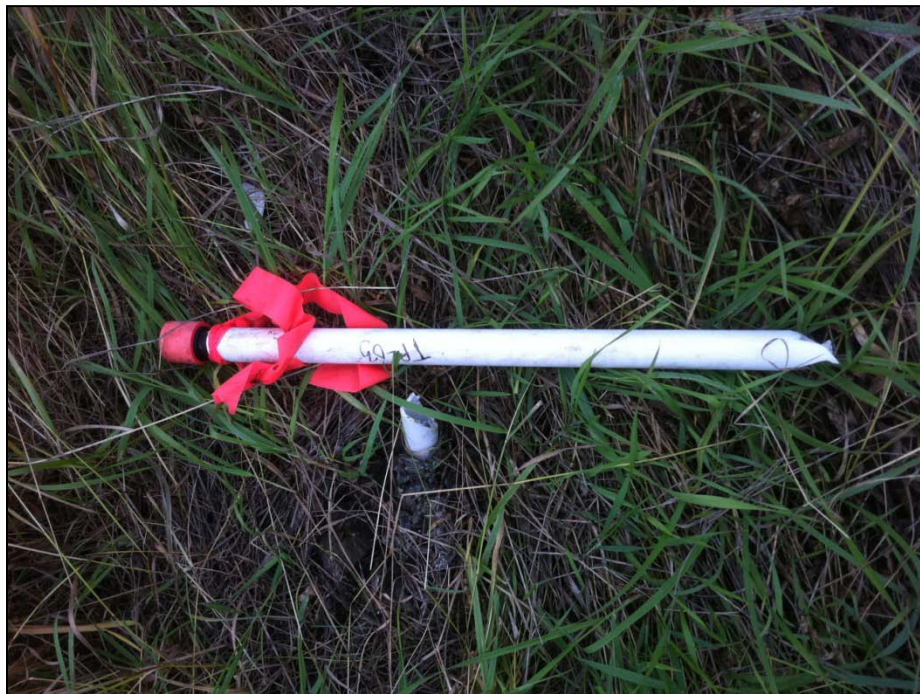
PHOTOGRAPH 6: VIEW OF TP-3 DESTROYED BY MOWER (SEPT 2011)
