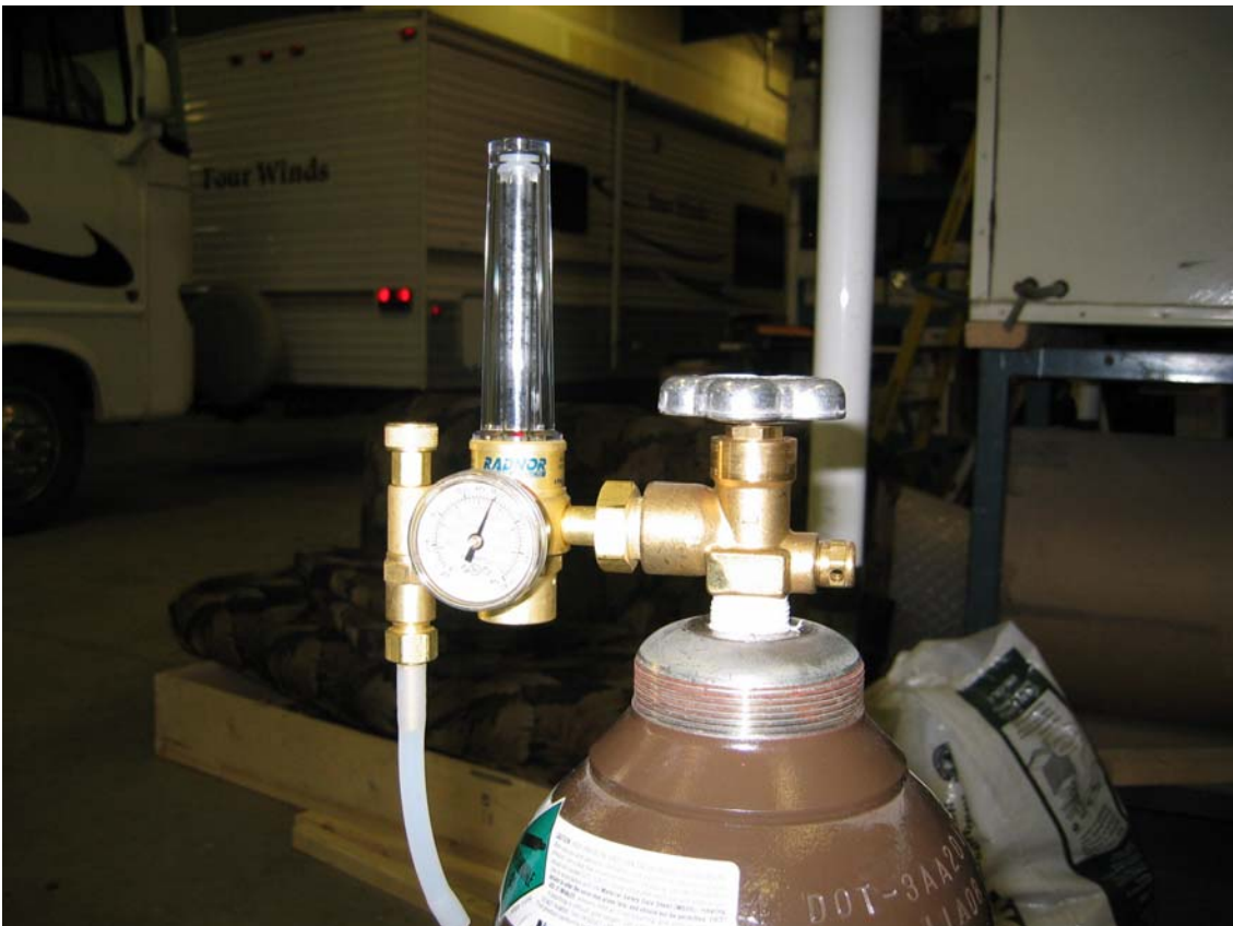
Photograph 4 Helium tank and regulator used in leak testing.
