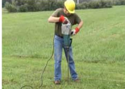
Rotary hammer drill with 36 inch long x 0.5 inch diameter carbide tipped bit
