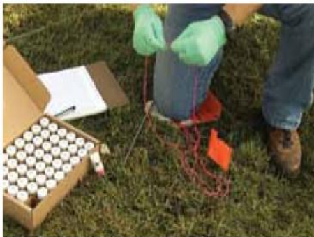
Cut 72 inch length of string and tie ends together to create loop.
