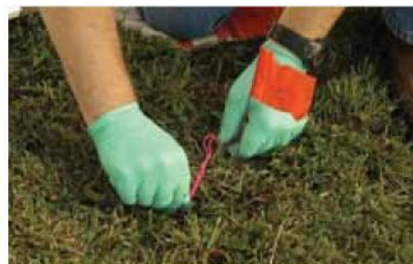
Push rod to the side and twist to detach sampler
