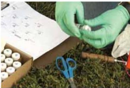
Attach tamper seal across cap and vial.
