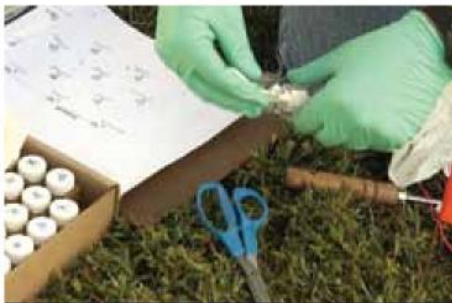
Return sampler to vial. Clean top of vial and threads and secure vial with cap.
