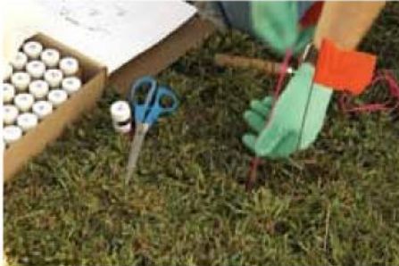
Pull string to remove sampler from hole
