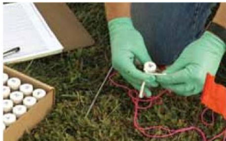
Match serial number of sampler with number on vial.
