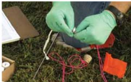
Loop string through looped end of sampler and secure.
