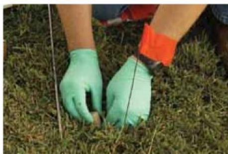
Insert cork to seal hole. (Rubber mallet may be necessary in sub-slab installations)
