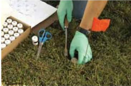
Remove cork by hand or with screwdriver
