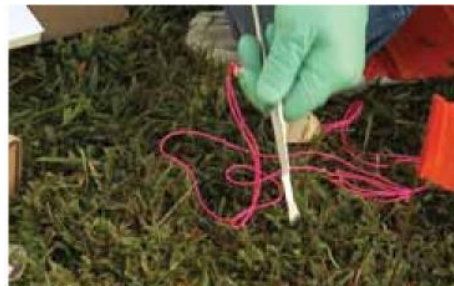
Place insertion rod into pocket of sampler.
