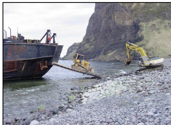
Photo 1. A bulldozer and excavator were required to help unload the remaining equipment from the barge.
