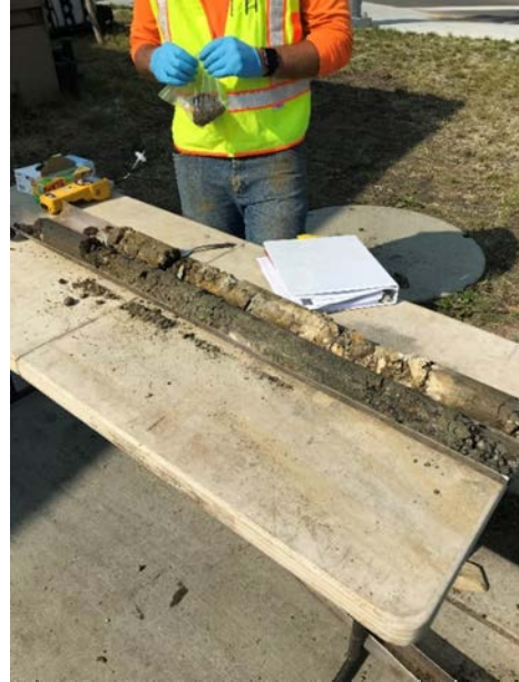
Photo 2: Representative soil boring samples extracted by macro-core with 5-foot disposable 1.6" diameter core sleeves, July 2019
