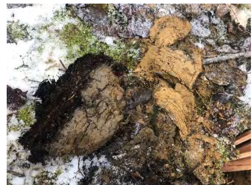
Exhibit 1: Comparison of native soil (left) with tailings (right) within the secondary tailings impoundment.
