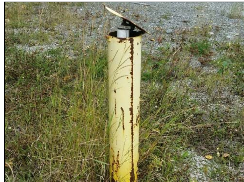
MWA22 PVC casing rising above out protective casing.
