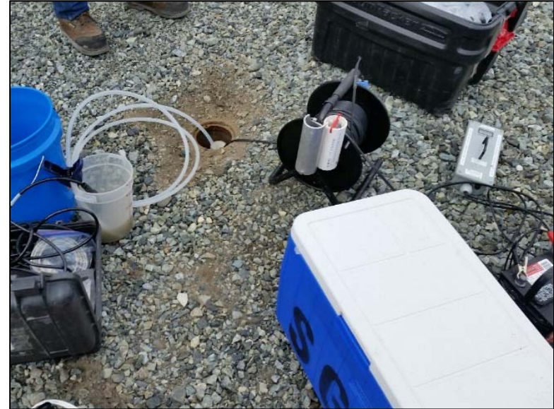
Sampling MWE06 using a submersible pump.
