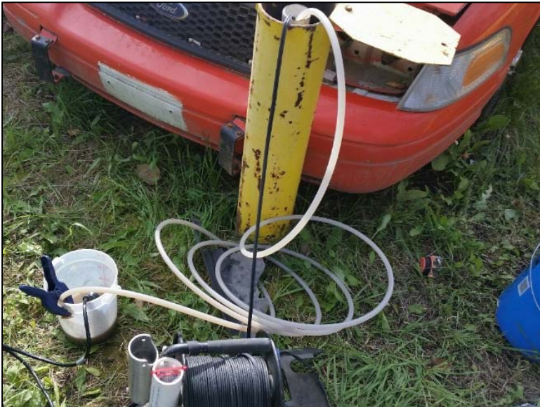
Sampling MWB17 using submersible pump.
