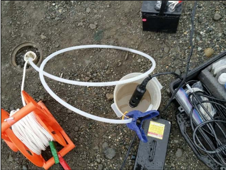
Sampling MWA05 using a submersible pump.
