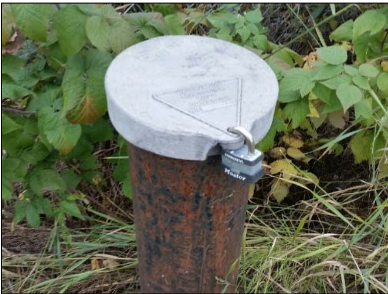
Locked outer protective casing of DPA32
