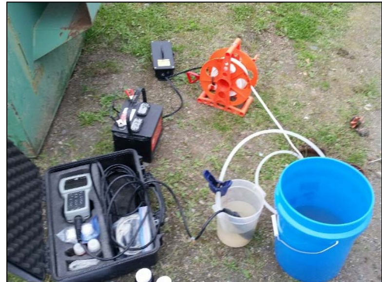
Sampling MWA07 using a submersible pump.
