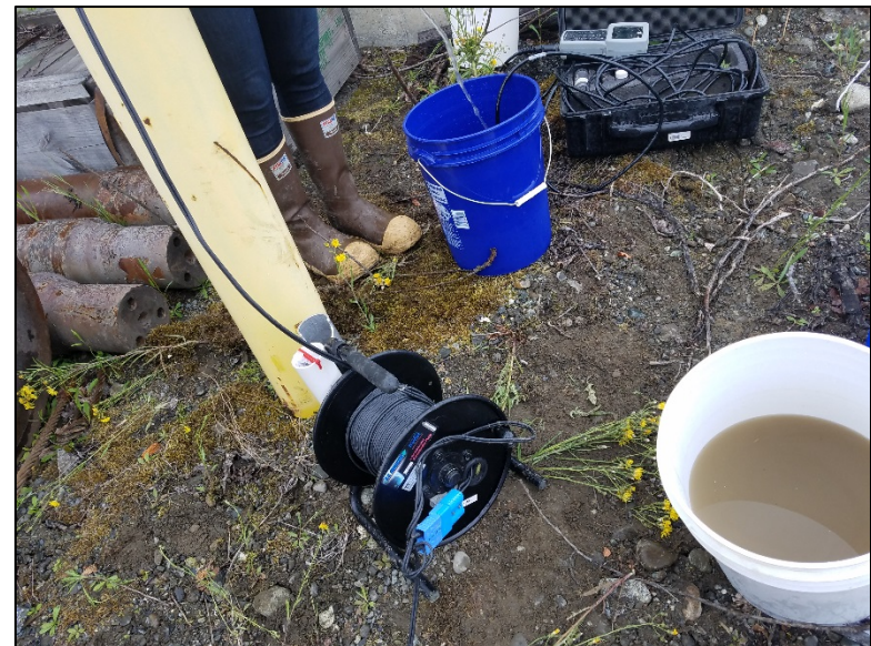
Sampling MWD01 with a submersible pump; purge water.
