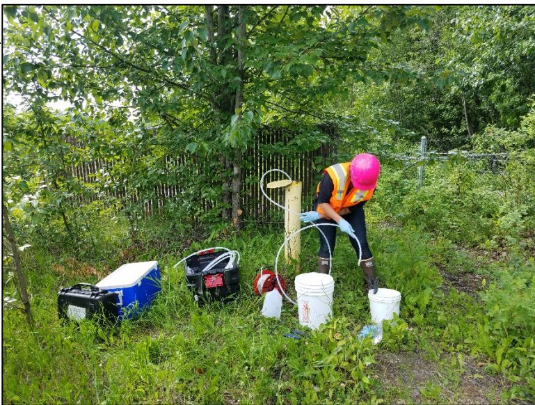
Sampling monitoring well MWB08 with a submersible pump; looking west.
