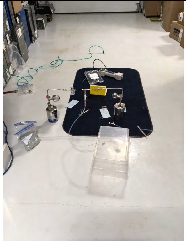
Sampling sub-slab soil gas with a duplicate T. Leak detection shroud in place. Tedlar bag used to measure soil gas adjacent to helium meter.
