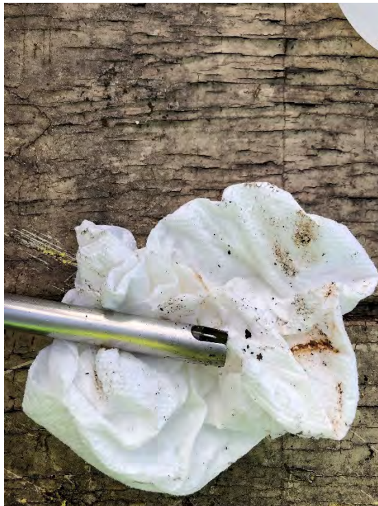
Photo 10: Rust in drinking water well found on the oil-water interface probe 11/15/19 11:41.
