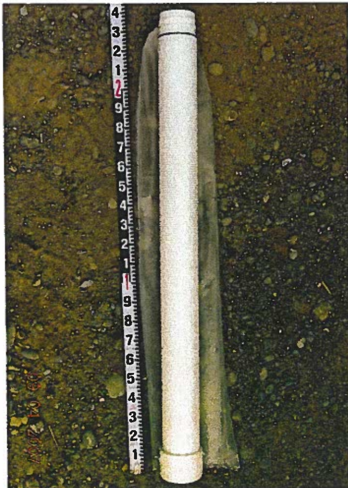
2 ft long x 2 in ID slotted PVC screen
