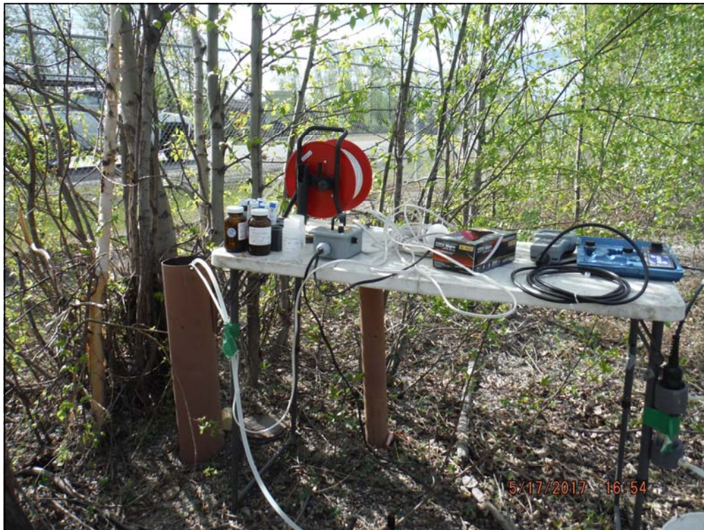
OU2 Building 1168—Groundwater sampling in AP-5751 (view W)
