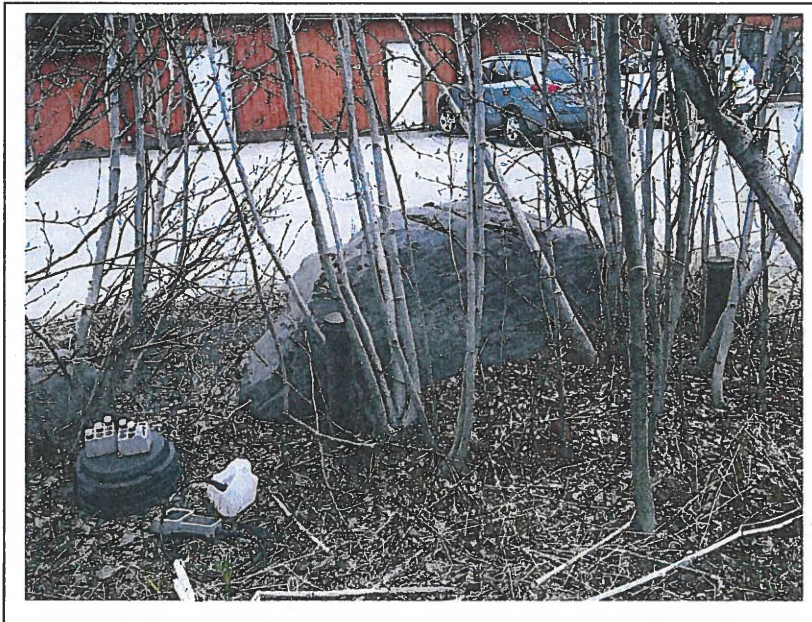
Photo4: Looking northeast, a view of the two standpipes for the buried UST. Samples were collected from the western standpipe on the left side in the photo. After the UST was sampled, purge water from the monitoring wells was poured into the UST (May 21, 2013).
