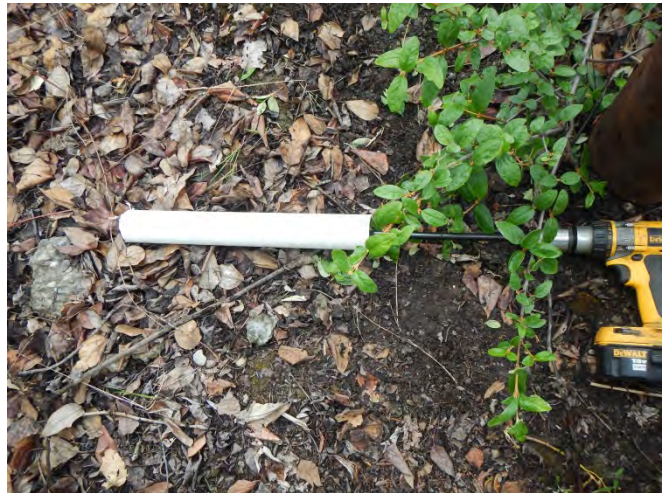
Removed portion of bent casing from MW-29.
