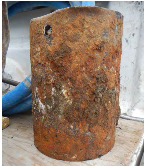
Metal casing removed from road at former MW-12 location.
