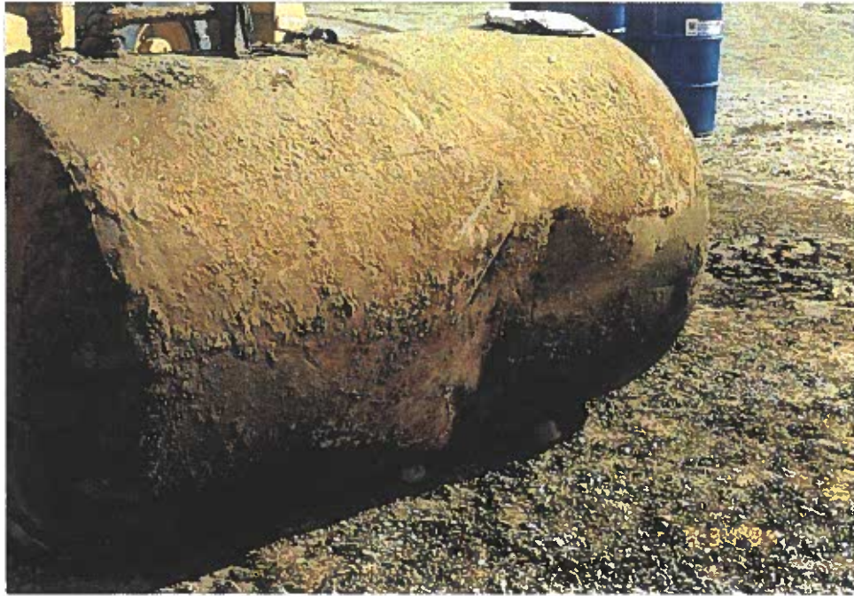
Photo 5: Several places were dented on UST No. 1 with no apparent punctures.
