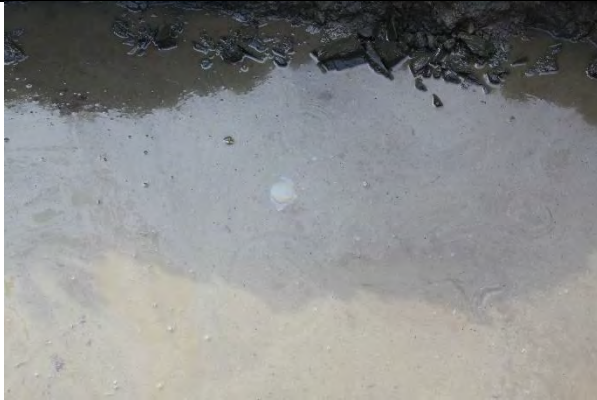
Photo showing petroleum sheen in groundwater of TH27.
