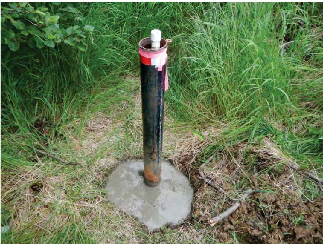
Photo 10: Site OT001, Subarea PT1, well PT1SB15; view of 2014 repaired condition.
