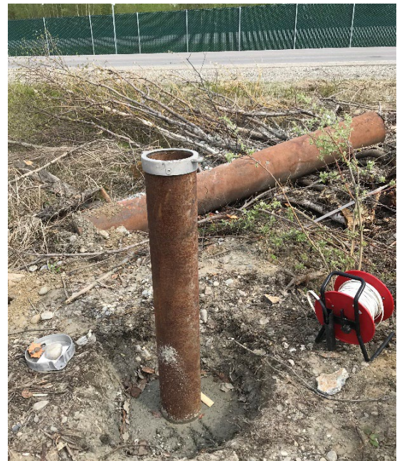
Exhibit 3-1: Measuring depth to groundwater at MW-30.
