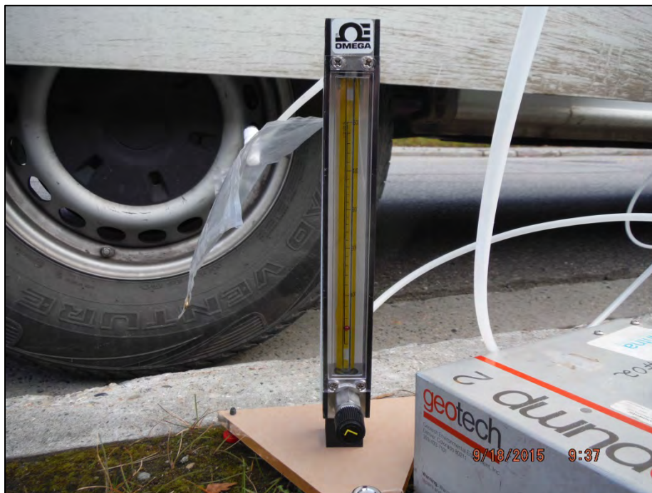
Photograph 8: Purging at 50 ml/min at VMP-4
