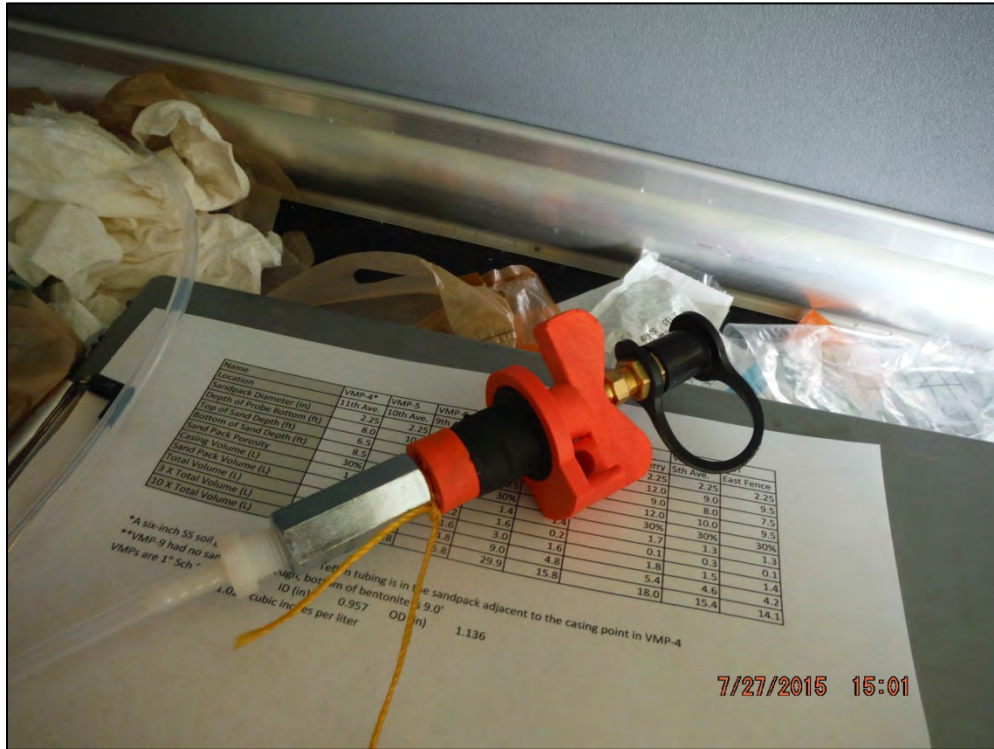
Photograph 3: Vapor Extraction Plug with Attached String and Teflon Tubing
