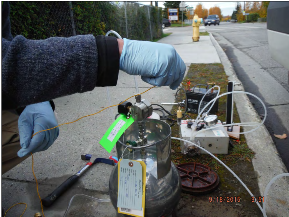
Photograph 10: Low Uptake Waterloo Membrane Sampler ® at VMP-5
