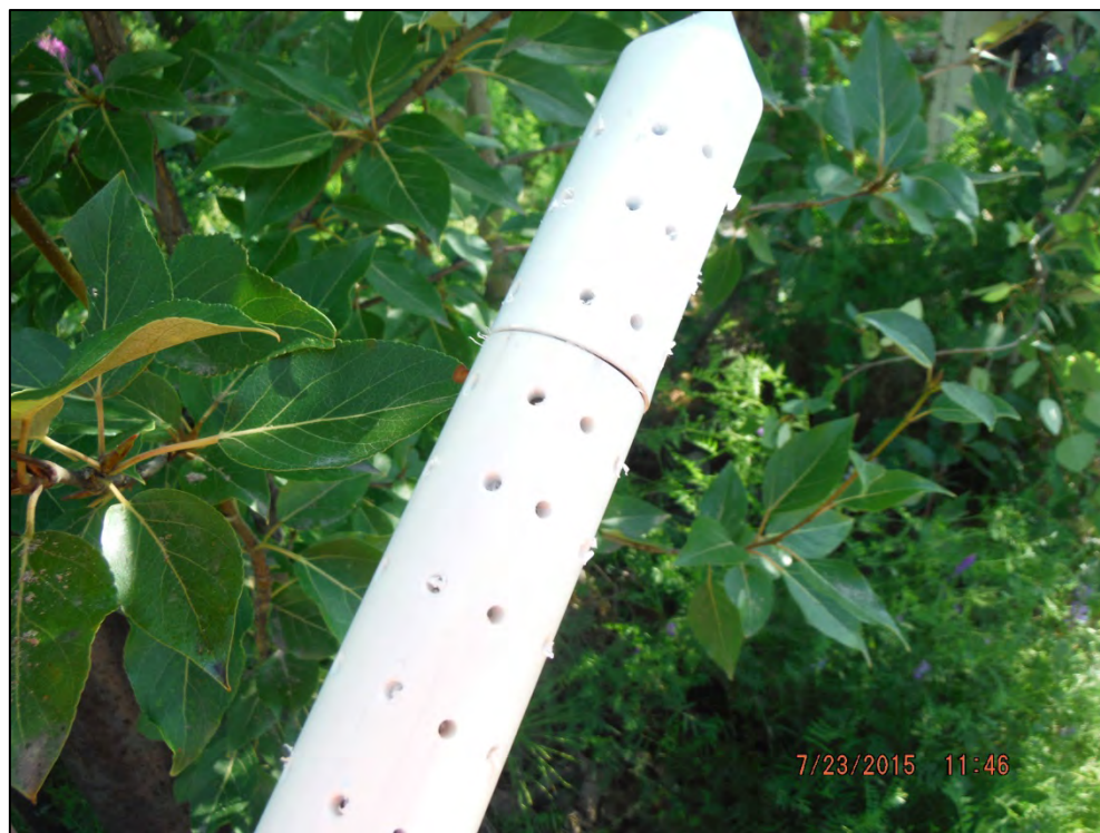
Photograph 2: 64 Perforations on Bottom Six Inches of VMP, 1/8-inch Diameter Each
