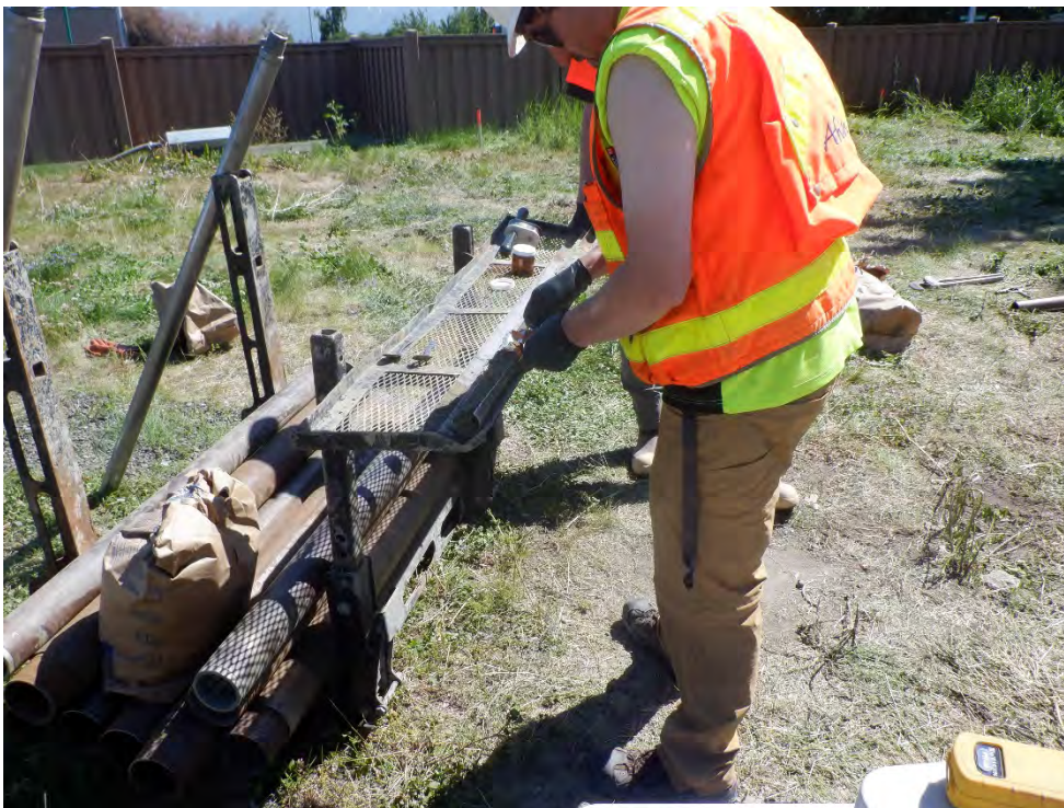
Photograph 12: Collecting soil analytical samples. View southeast.
