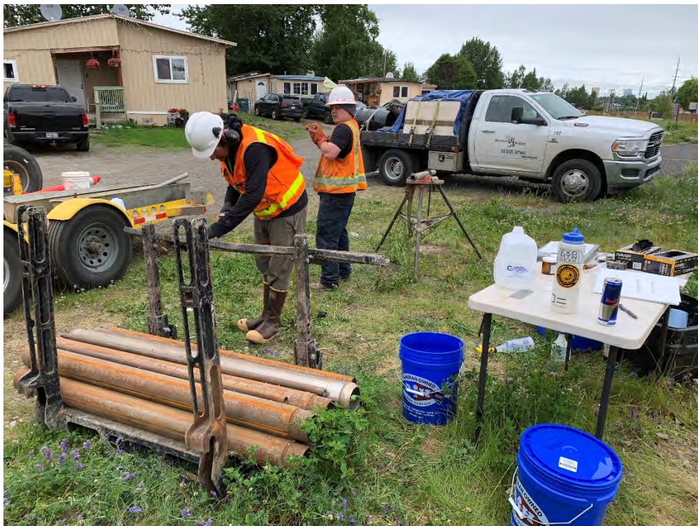
Photograph 6: PID screening soils. View north.
