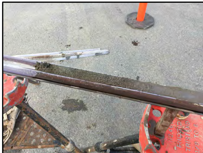
PHOTO 7 - LITHOLOGICAL CHANGE OBSERVED AT MW-4 (25-26 FBG)
