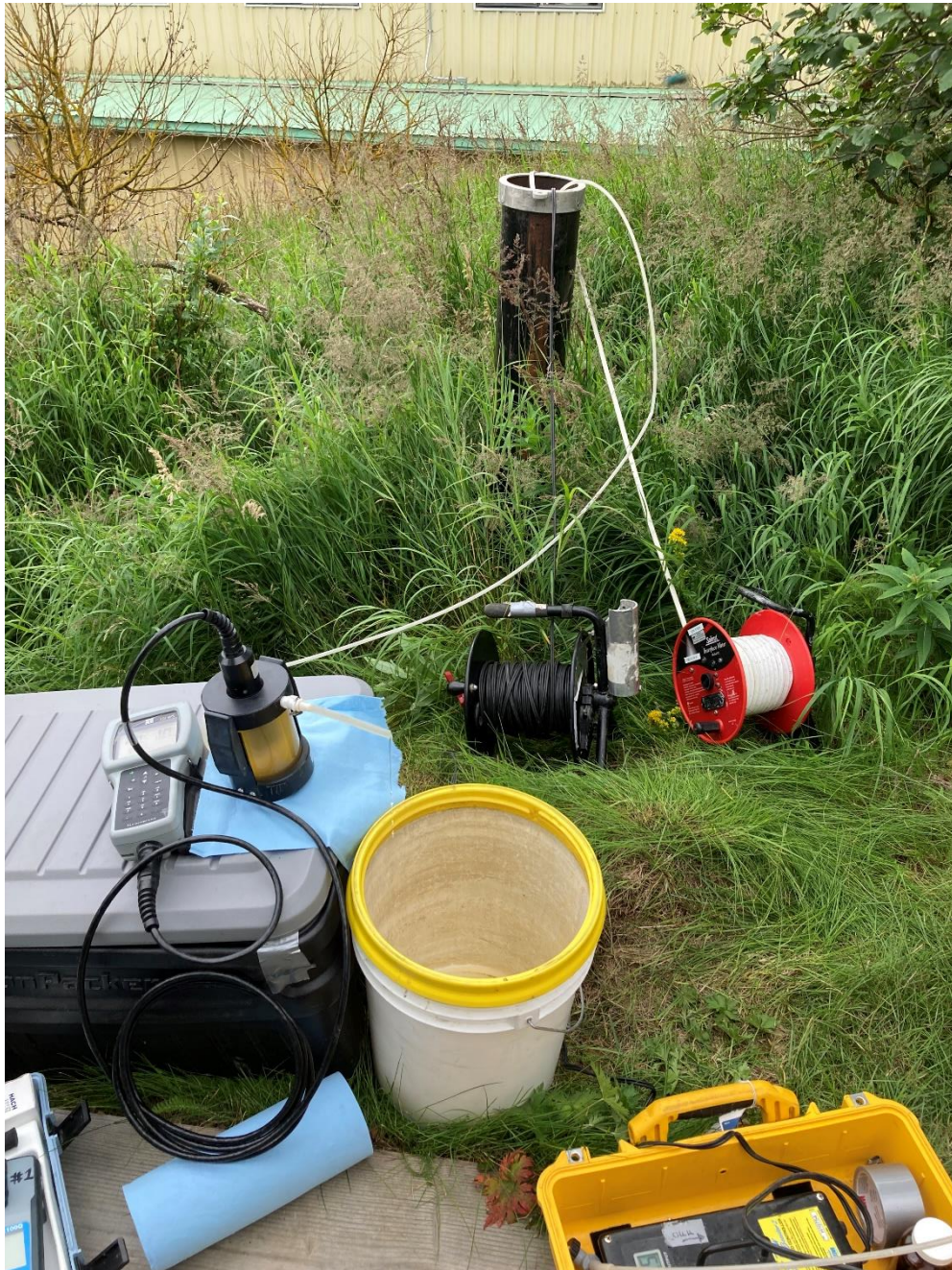
Photo 2: Monitoring Well 6 sampling set up.
