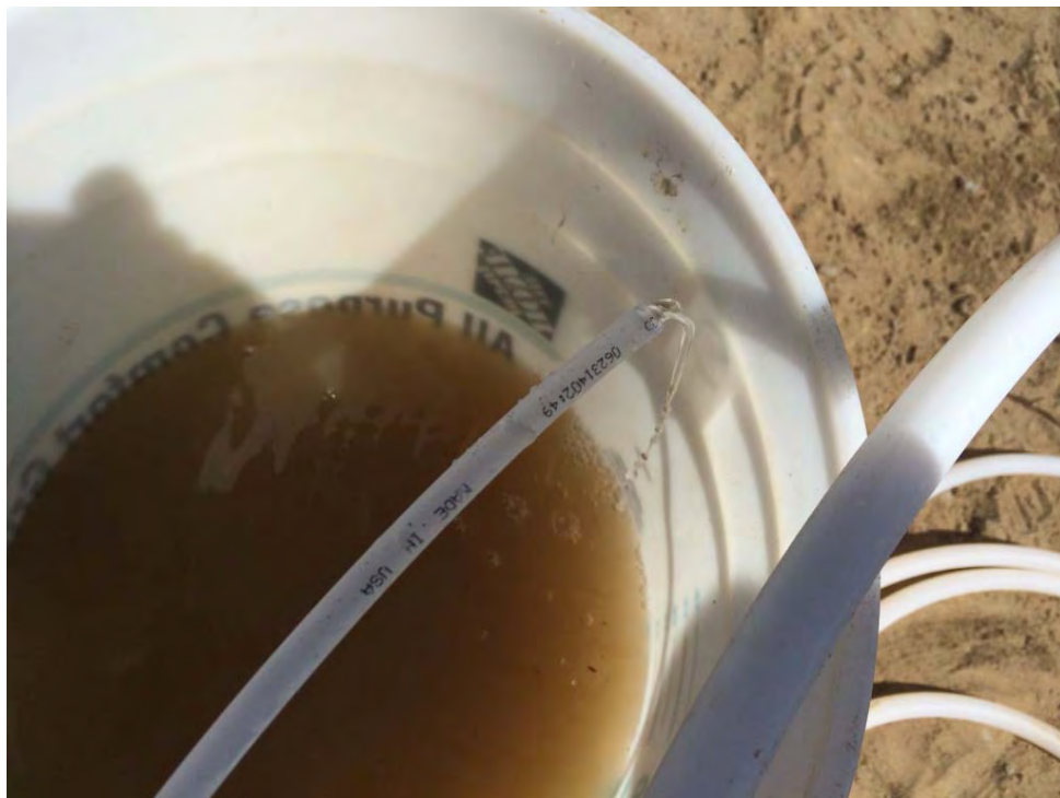
Photo 12: Monitoring wells were surged and purged to remove sediment until purge water was visibly clear.
