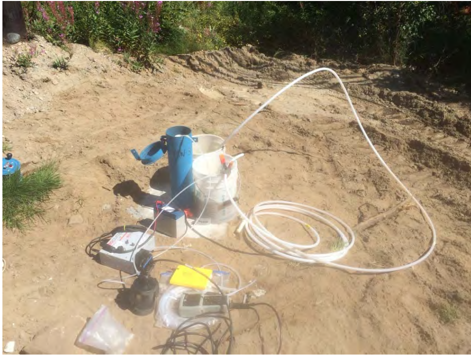
Photo 11: Sampling monitoring well MW-3 after developing with surge block.
