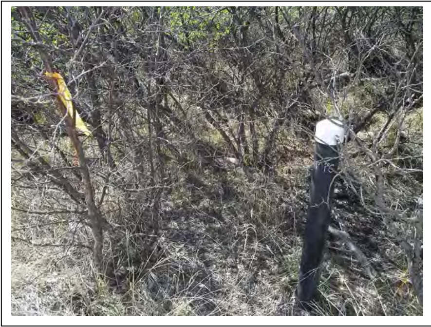
Photo 13: Monitoring Point MPC was viable, but sediment or debris in the well was above the screen interval. (May 12, 2014)
