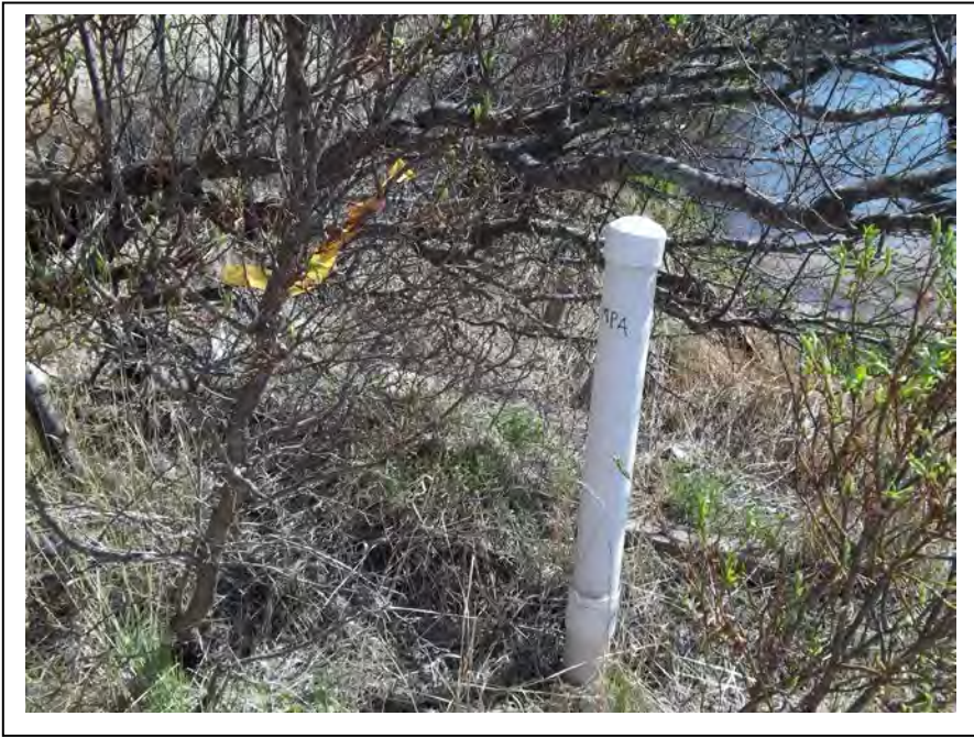
Photo 11: Monitoring Point MPA was dry and filled with sediment above the screened interval. (May 12, 2014)
