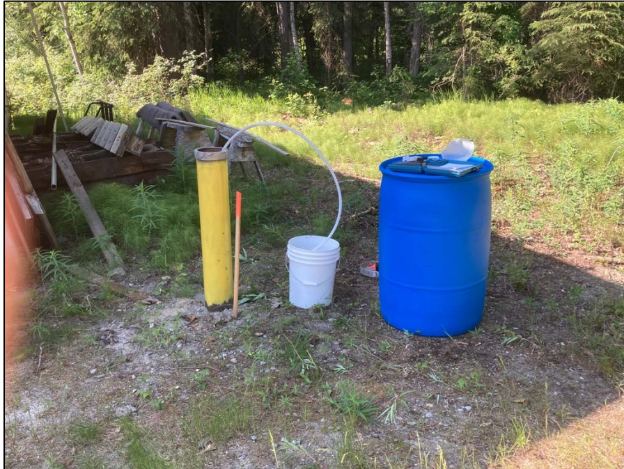
Photo 3. Well development at MW-3 facing south. June 16, 2022
