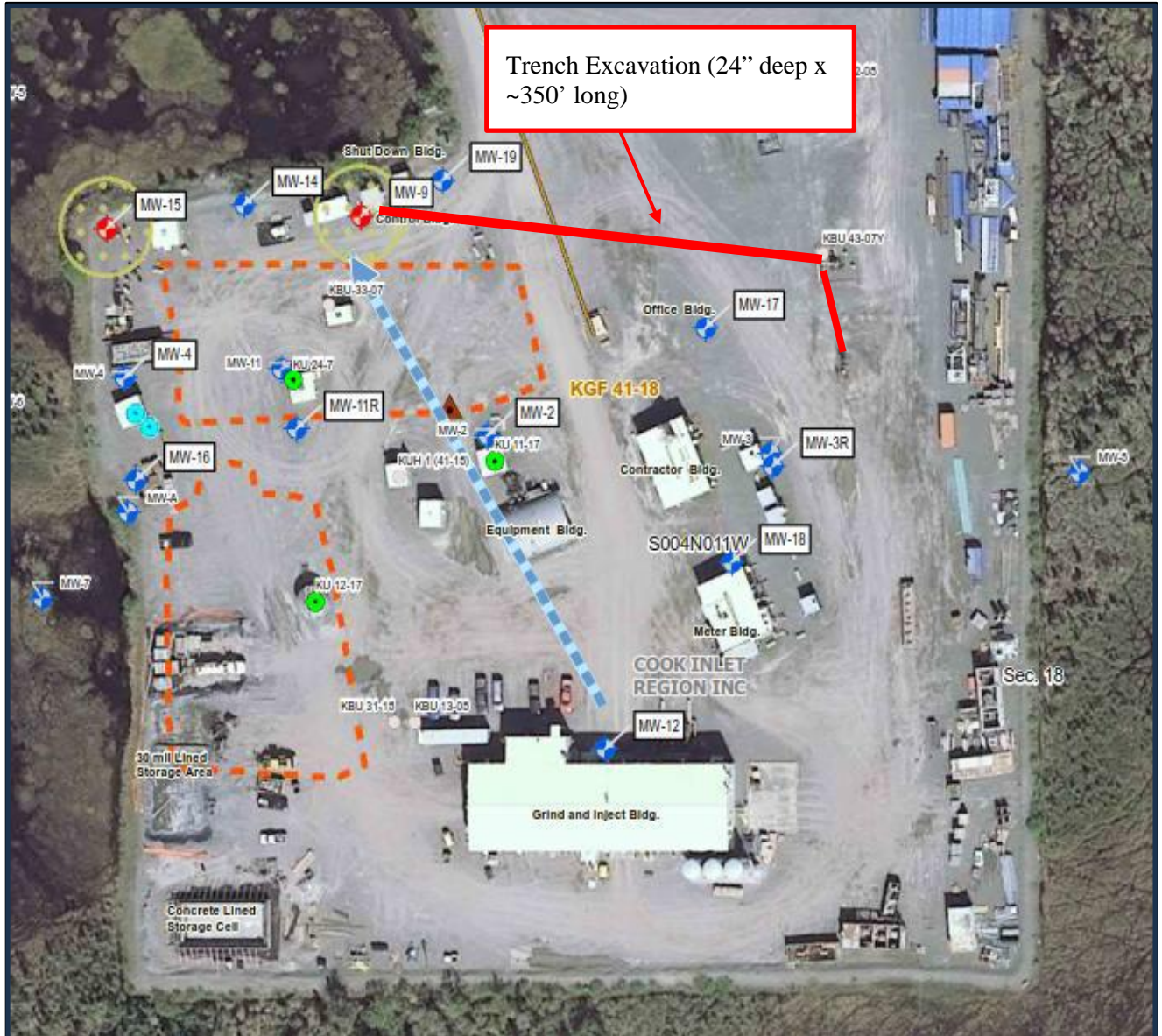
Soil Management Plan for Trench Excavations, Kenai Gas Field 41-7 and 41-18 Facilities
