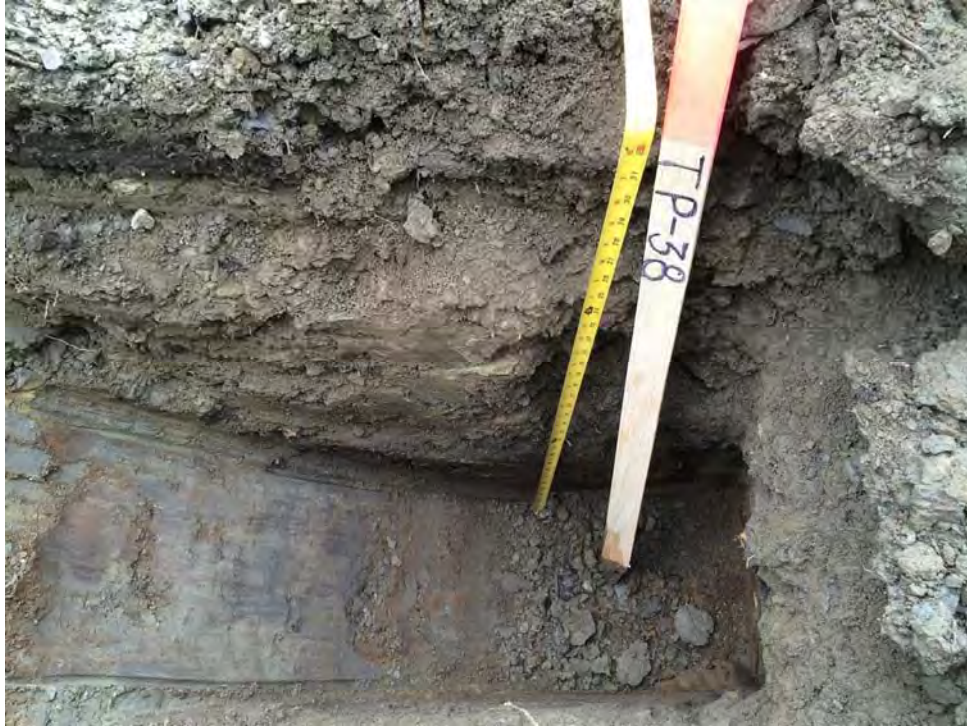
Photo 3 - Soil profile at TP-38 - new coarse material overlying silt and gravel mix overlying native silt.
