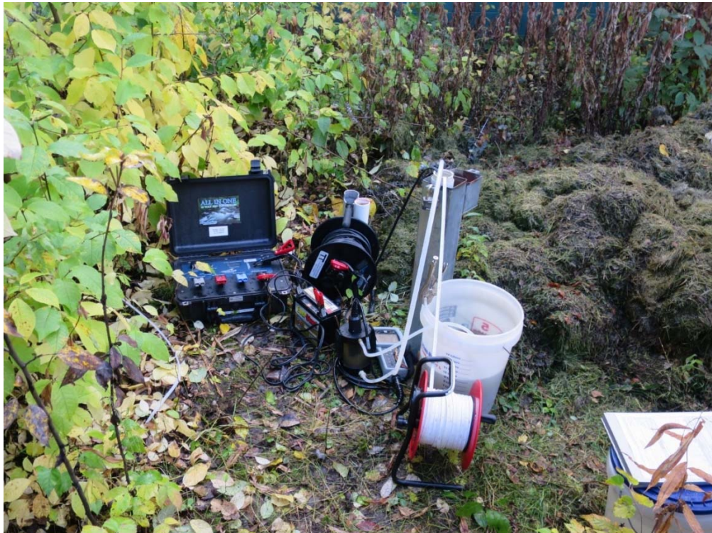
Photo 2: Monitoring well MW-3 during purging.
