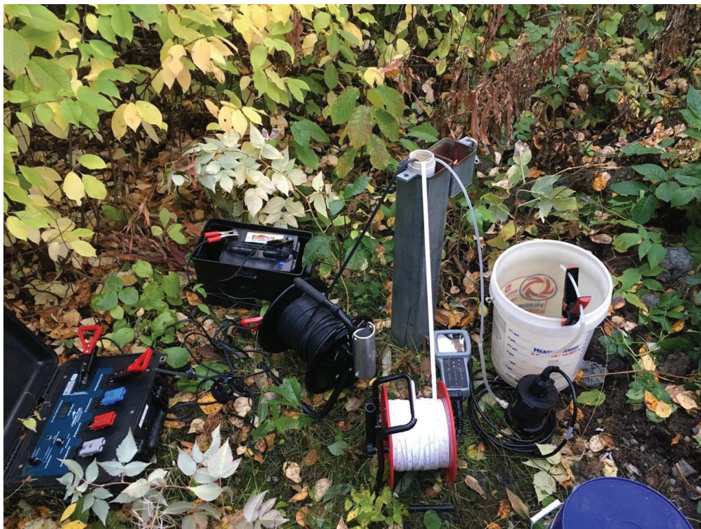
Photo 2: Monitoring well MW-3 during purging.
