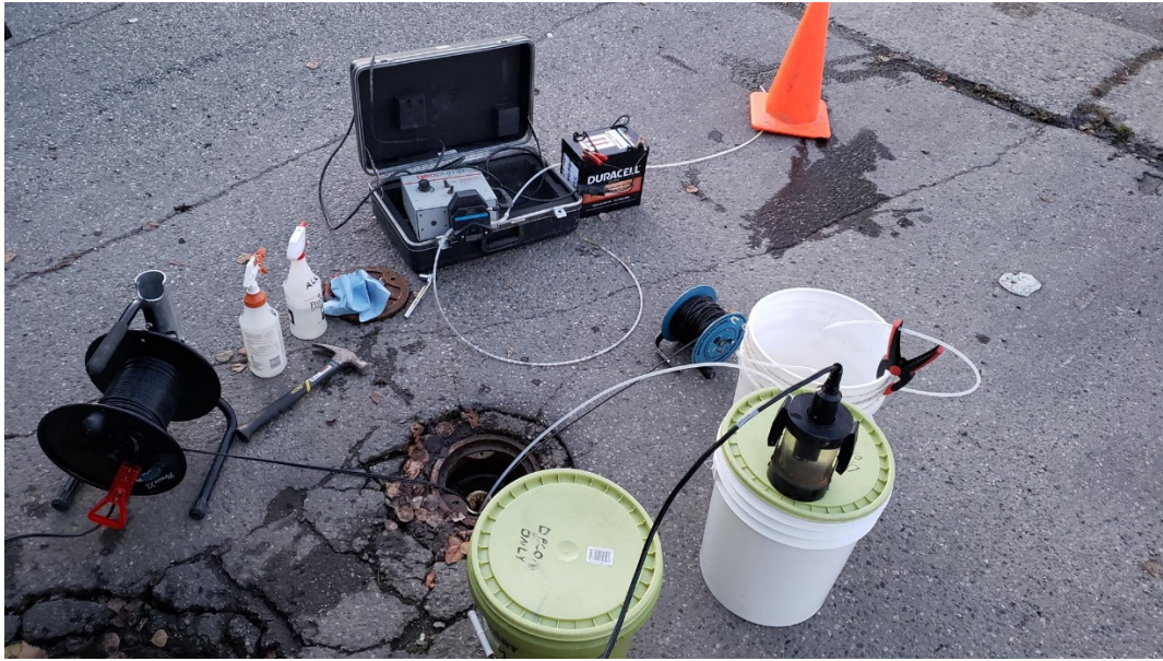
Photo 1: Monitoring well MW-34A during purging following removal of water from monument.
