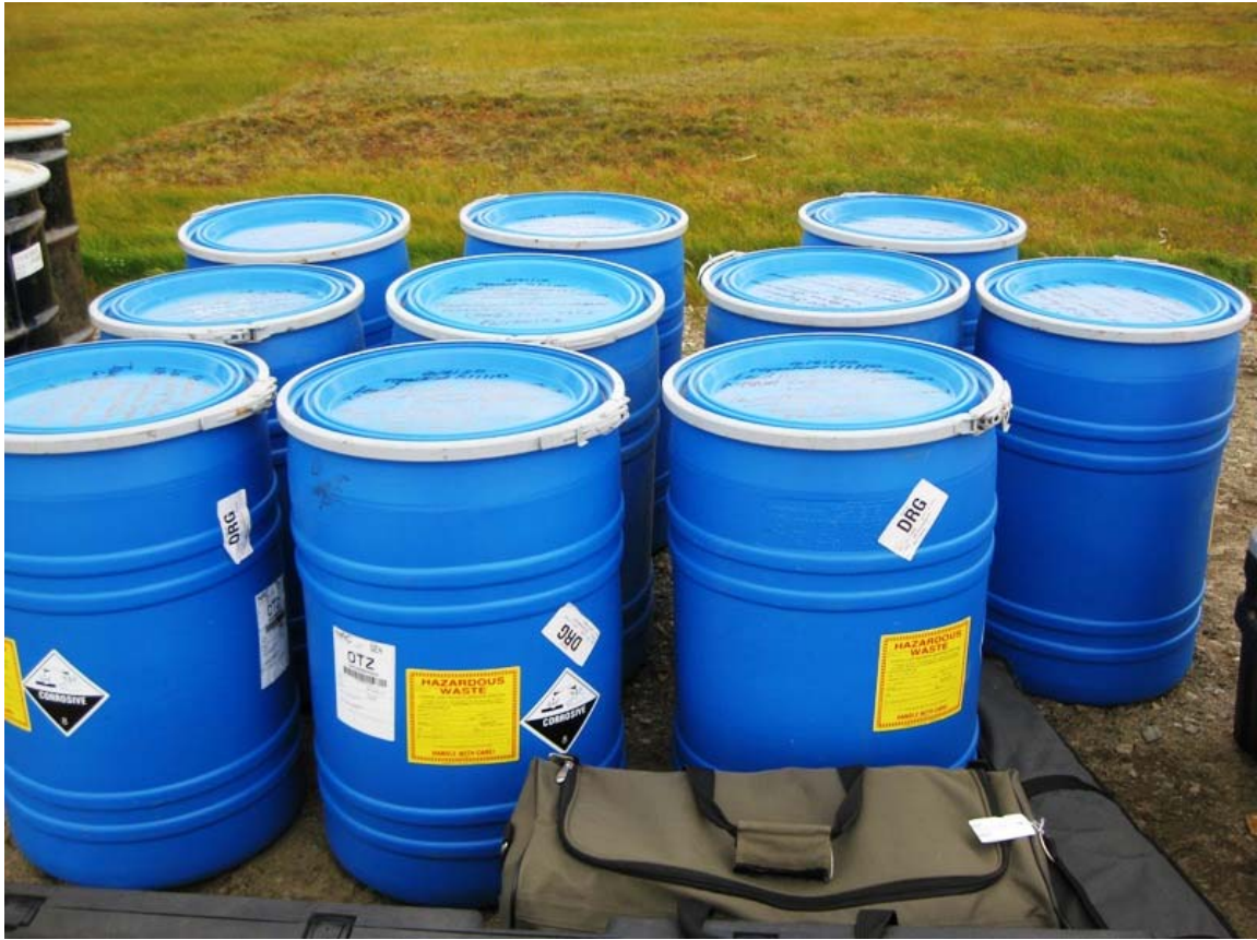
3. Polyethylene drums containing lead-acid batteries for transport to a disposal facility.
