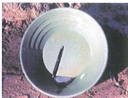
Figure 2. Gold pan with more than 30 grams of mercury from 1 kilogram of mercury-contaminated sediments.
