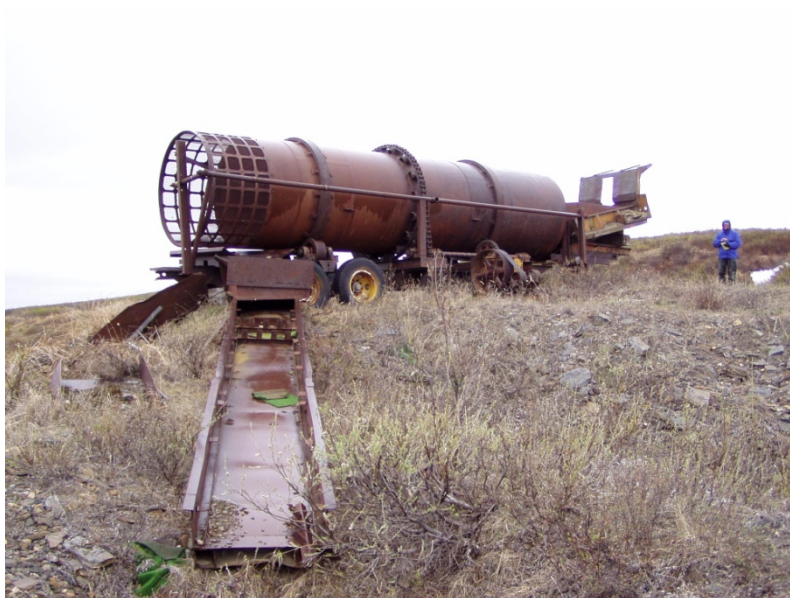
16. Photo copied from SLR 2005 Phase I ESA. SLR identified this piece of equipment as a roller mill. This is a gold recovery trommel and is used like a screen and as the main drum portion of the trommel rotates it mechanically separates coarse material from fine grained material. Water is introduced in the upper portion of the trommel which catches the fines to transport them along the sluice for gold recovery. There is no crushing or grinding involved with the use of gold recovery trommels.
