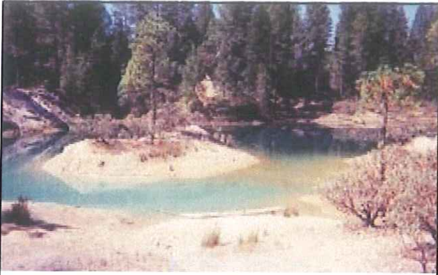
Lake in hydraulic mine pit caused by blocked drainage tunnel. Acidic water in this pit lake (pH 3.5) caused by oxidation of sulfide minerals in gold-bearing gravel deposits.
