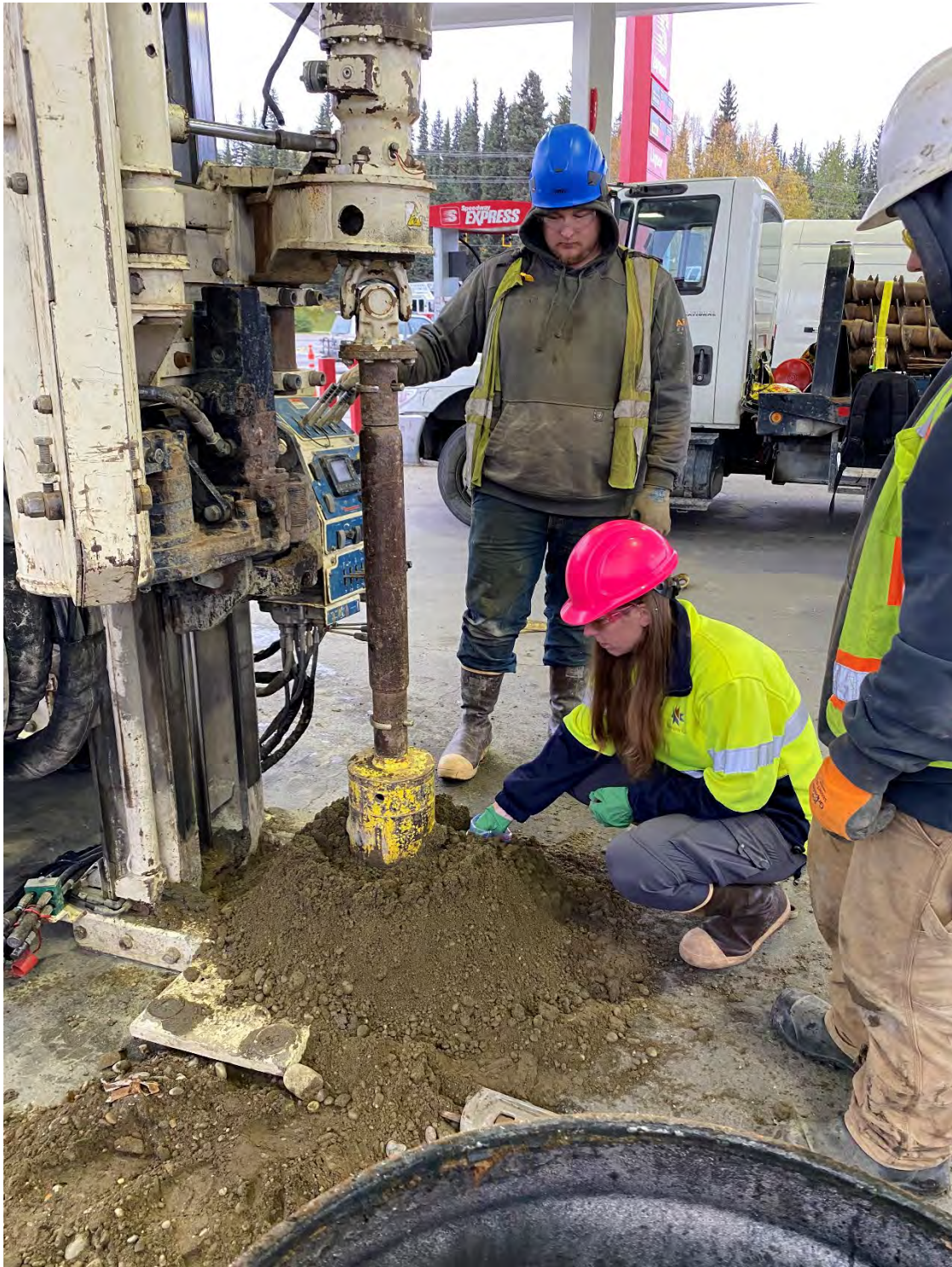
Photo 6: Taking soil samples of IW-2023-C.
