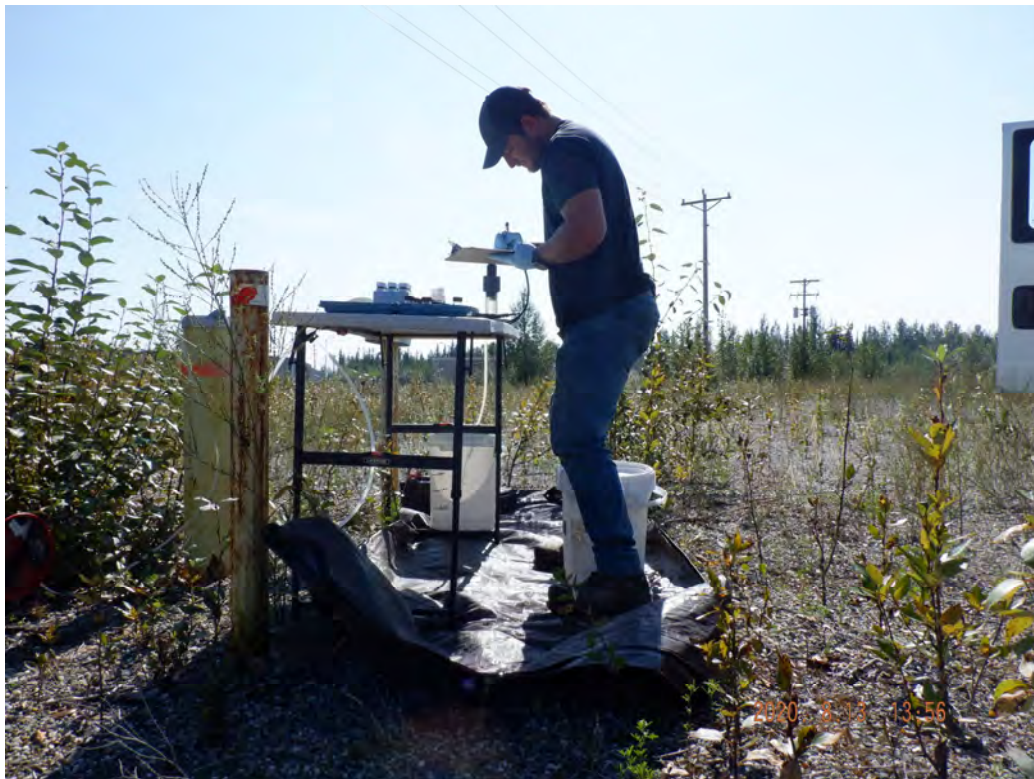
Collecting groundwater parameters while purging monitoring well AP-10015R (view SE)
