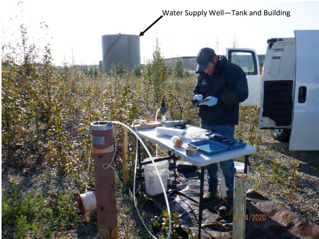
Collecting groundwater parameters while purging monitoring well AP-10016R. Water Supply Well building in background (view SE)
