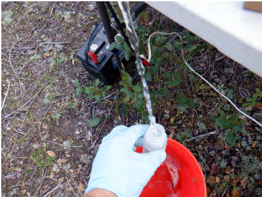
Collecting a groundwater sample at AP-8916 (view NA)
