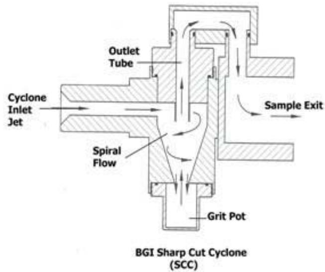
**Figure 1-1 Particulate flow path through PM 2.5 Sharp Cut Cyclone**
