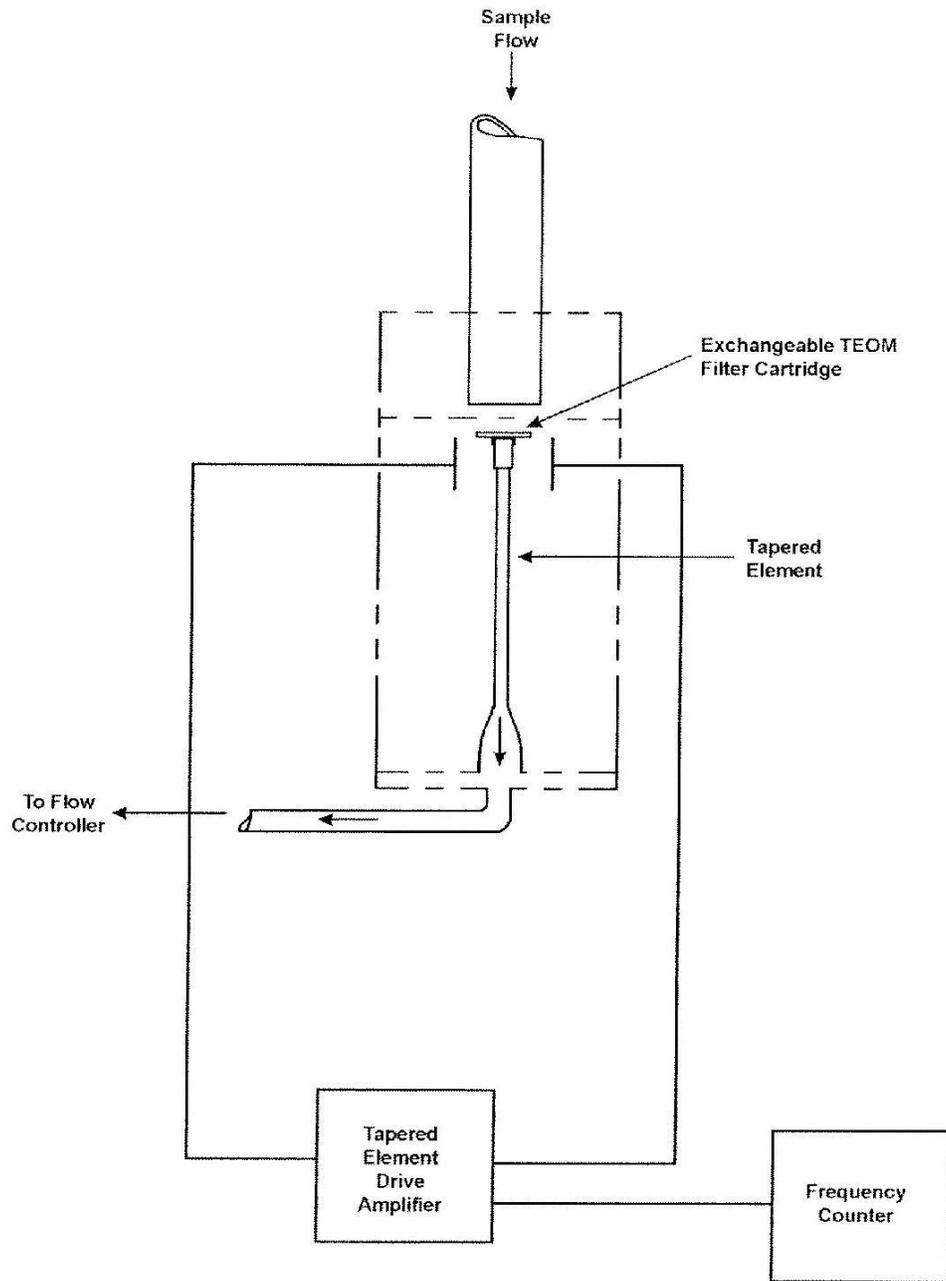
**Figure 1-2 Schematic Diagram of Mass Transducer**
