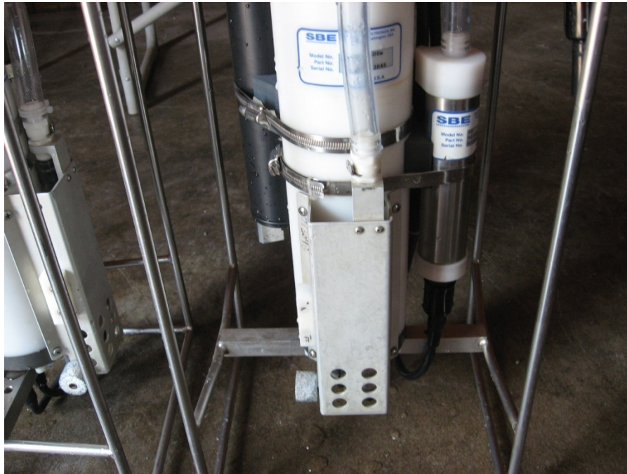
Figure 3. Sea-Bird SBE-19 CTD Sensor with Integrated SCUFA® Fluorometer
