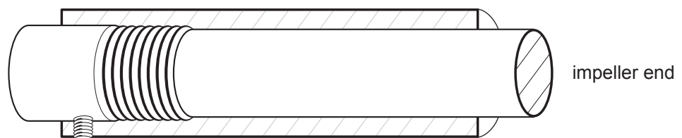
Shaft sleeve threaded to shaft
