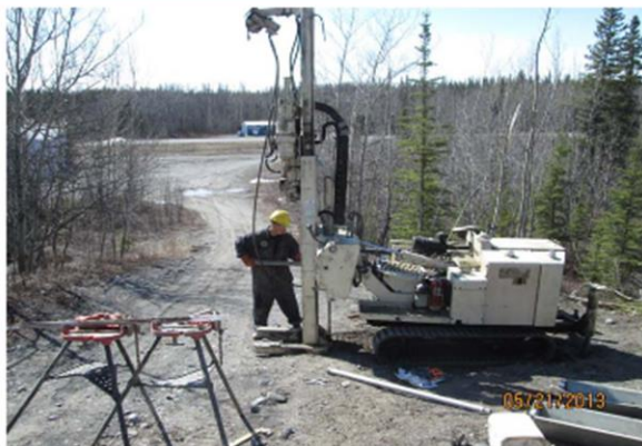
A drill rig takes soil samples at a site in Glennallen, Alaska targeted for reuse as the home for a new fire station. Environmental sampling is one of the many services that applicants are eligible for through the DBAC program.
