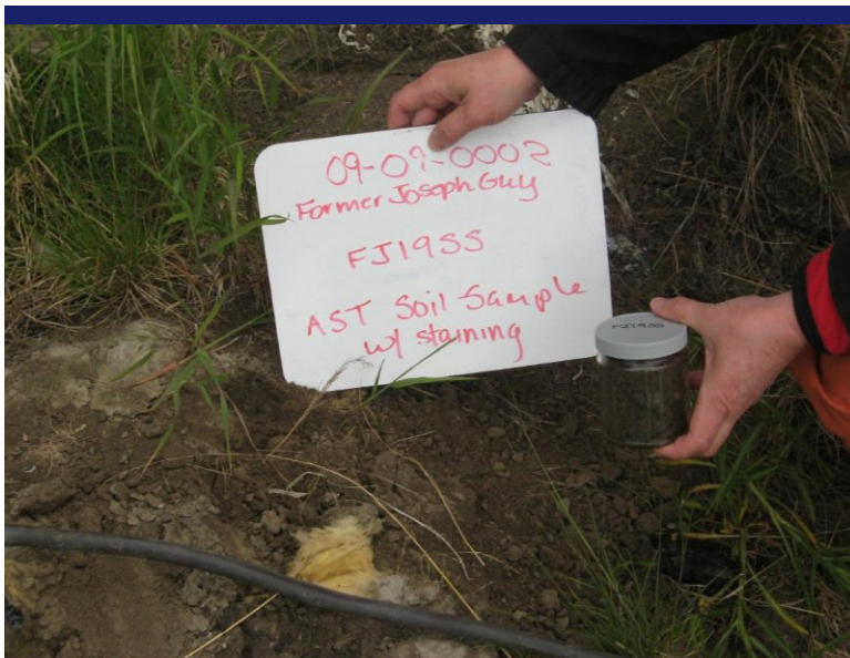
Photo 3 Sample FJ19SS, an oil-stained soil sample collected near the former AST location.
