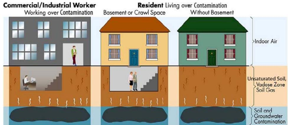
Contamination in the soil and groundwater can take the form of a vapor and travel through soil, entering indoor air through leaks in parts of buildings which are below-ground, like basements and crawl spaces.
