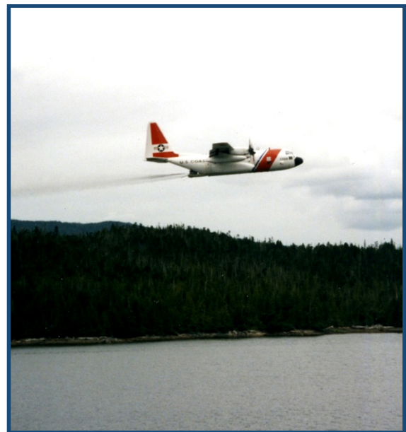
Test of aircraft dispersant application equipment during CANUSDIX drill. (ADEC Photo)
