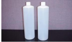
**Get a Sample Kit From Your Lab** – Contact the lab for sample bottles. The lab will send the proper plastic sample bottles for collecting the samples.
