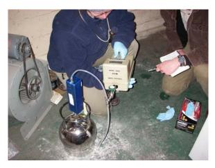
Once time is given for the cement to cure, the sample can be collected. Sub-slab samples are typically collected over a 20 to 30 minute timeframe.
